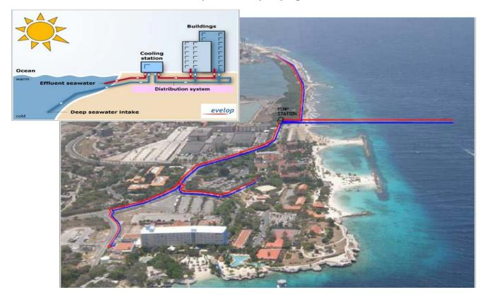
Rationale: Aqualectra/Evelop planned to engineer and build a Sea Water Air Conditioning for hotels in the Piscadera area. This air conditioning makes use of the cold sea water from a depth of about 800 meter. The deep sea water contains high concentrations of nutrients. The disposal of this cold, nutrient rich water may cause serious problems, like algae growth.
