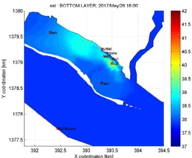
Rationale: The goal of the project was to investigate the current brine dispersion in the lagoon and to give recommendations for optimization of the brine disposal. The main aspect is to prevent the possible occurrence of a stratified situation in the lagoon, especially during low wind season, since the occurrence of a layer of brine (stratified situation), which hardly dilutes and spreads over a large area, negatively affects benthic flora and fauna.
